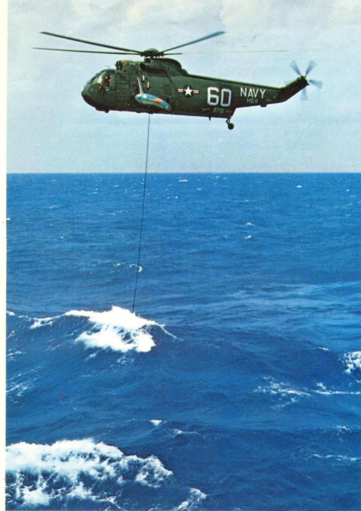
Sonar designed for submarine detection is dunked into the sea by a U.S. Navy/Sikorsky S-61 Sea King, an anti-submarine weapons system capable of searching out, identifying, tracking, and destroying undersea craft. Sea Kings have been ordered by the governments of the United States, Canada, England, Italy, Spain, and Japan.
