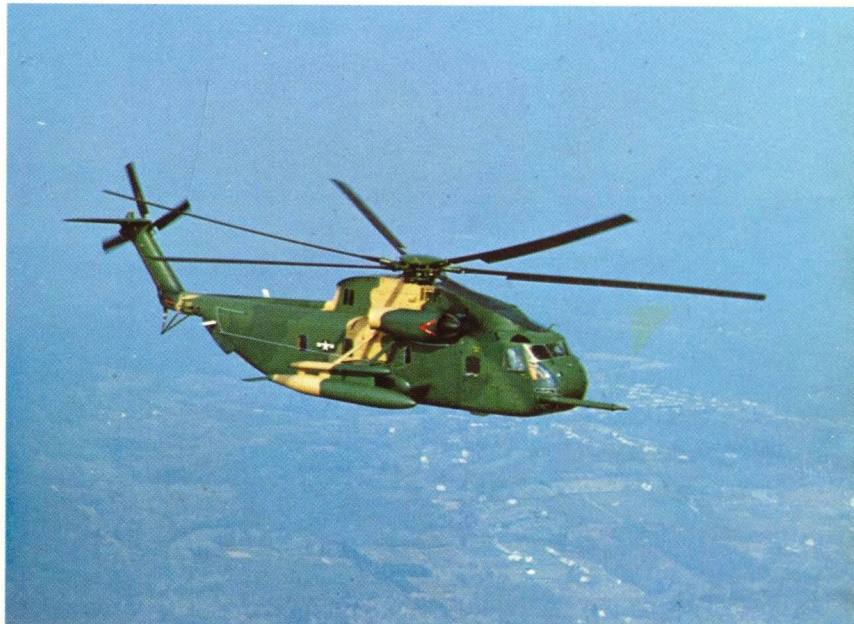
The U.S. Air Force's largest and fastest helicopter is the Sikorsky S-65, a long-range aircraft used by the Aerospace Rescue and Recovery Service. Like the Sikorsky S-61R, the S-65 is equipped for aerial refueling from a Lockheed C-130 tanker/transport to extend its range to the limit of its flight crew's endurance.
